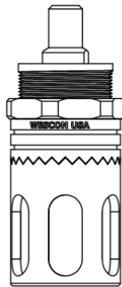
WES296-SL-S Microstop with Ø 1/4" Standard Shaft
