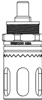
WES296-SL-S Microstop with Ø 1/4" Standard Shaft
