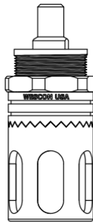
WES296-SL-S Microstop with Ø 1/4" Standard Shaft
