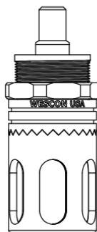
WES297-SL-S Microstop with Ø 1/4" Standard Shaft
