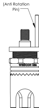
WES297-S3L-TS-AR Microstop with 1/4-28 Threaded Shank Shaft and Anti Rotation Pin
