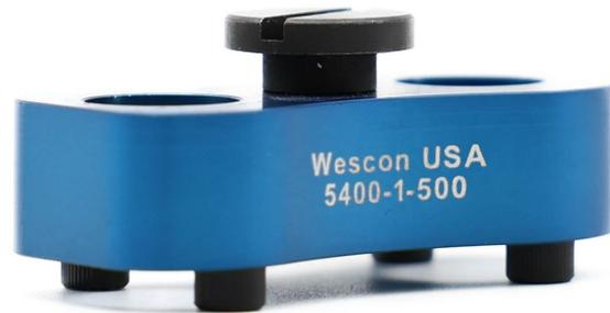
SR Type Dog Bone Drill Guide - used to guide drill in hand held drilling applications. Ergonomic design for superior positioning and alignment in order to drill perpendicular to the work surface. Nylon feet on each drill block to protect the drilling surface. Made from anodized aluminum for increased durability and wear resistance. To be used with standard slip/fixed type renewable drill bushings (sold separately).
