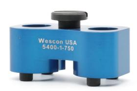
SR Type Dog Bone Drill Guide - used to guide drill in hand held drilling applications. Ergonomic design for superior positioning and alignment in order to drill perpendicular to the work surface. Nylon feet on each drill block to protect the drilling surface. Made from anonized aluminum for increased durability and wear resistance. To be used with standard slip/fixed type renewable drill bushings (sold separately).
