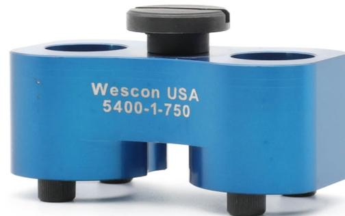
SR Type Dog Bone Drill Guide - used to guide drill in hand held drilling applications. Ergonomic design for superior positioning and alignment in order to drill perpendicular to the work surface. Nylon feet on each drill block to protect the drilling surface. Made from anodized aluminum for increased durability and wear resistance. To be used with standard slip/fixed type renewable drill bushings (sold separately).
