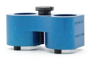
SR Type Dog Bone Drill Guide - used to guide drill in hand held drilling applications. Ergonomic design for superior positioning and alignment in order to drill perpendicular to the work surface. Nylon feet on each drill block to protect the drilling surface. Made from anonized aluminum for increased durability and wear resistance. To be used with standard slip/fixed type renewable drill bushings (sold separately).
