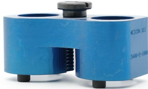
SR Type Dog Bone Drill Guide - used to guide drill in hand held drilling applications. Ergonomic design for superior positioning and alignment in order to drill perpendicular to the work surface. Nylon feet on each drill block to protect the drilling surface. Made from anodized aluminum for increased durability and wear resistance. To be used with standard slip/fixed type renewable drill bushings (sold separately).
