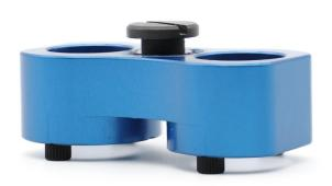
SR Type Dog Bone Drill Guide - used to guide drill in hand held drilling applications. Ergonomic design for superior positioning and alignment in order to drill perpendicular to the work surface. Nylon feet on each drill block to protect the drilling surface. Made from anonized aluminum for increased durability and wear resistance. To be used with standard slip/fixed type renewable drill bushings (sold separately).
