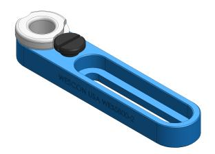
The WES5800 is a high-precision adjustable drill bar made in the USA from anodized aluminum. It holds ½" or ¾" slip or fixed drill bushings securely, delivering clean, accurate holes every time. This tool, also known as a "snatch block" or "steam boat", is ideal for hole repair, reaming, and aligning fastener holes in aircraft sheet metal. Lightweight and easy to handle, it lets you line up the drill perfectly over existing or misaligned holes.
