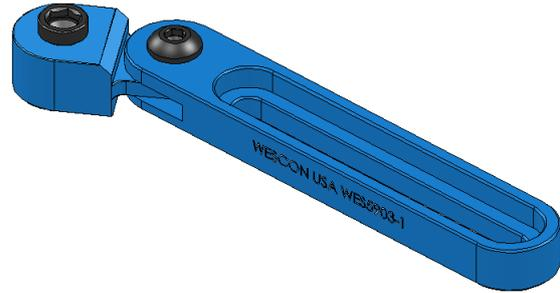
The WES5903 has a left-right swivel head for precise drilling over offset or angled holes. It works with WES5501 / 3/8-16 OD and WES5502 / 1/2-13 OD threaded bushings, giving flexibility without sacrificing stability. This high-precision adjustable drill bar, also known as a "snatch block" or "steam boat", is made in the USA from anodized aluminum. Perfect for aircraft sheet metal repair, structural hole alignment, and maintenance tasks where accuracy is critical.
