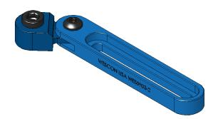
The WES5903 has a left-right swivel head for precise drilling over offset or angled holes. It works with WES5501 / 3/8-16 OD and WES5502 / 1/2-13 OD threaded bushings, giving flexibility without sacrificing stability. This high-precision adjustable drill bar, also known as a "snatch block" or "steam boat", is made in the USA from anodized aluminum. Perfect for aircraft sheet metal repair, structural hole alignment, and maintenance tasks where accuracy is critical.
