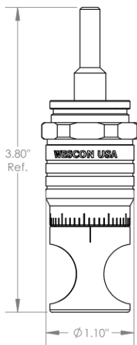
WES596-S Microstop with Ø 1/4" Standard Shaft
