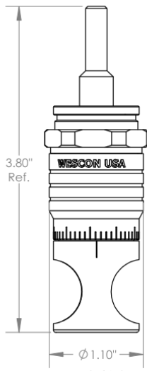
WES596-S Microstop with Ø 1/4" Standard Shaft
