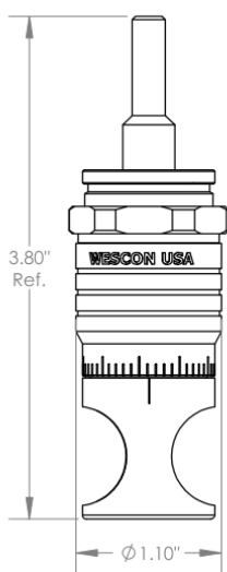
WES596-S Microstop with Ø 1/4" Standard Shaft
