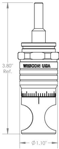
WES596-S Microstop with Ø 1/4" Standard Shaft
