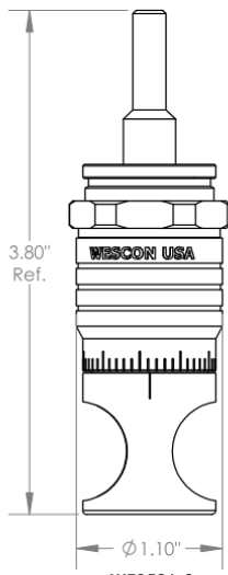
WES596-S Microstop with Ø 1/4" Standard Shaft
