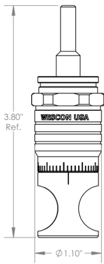
WES596-S Microstop with Ø 1/4" Standard Shaft
