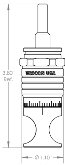
WES596-S Microstop with Ø 1/4" Standard Shaft
