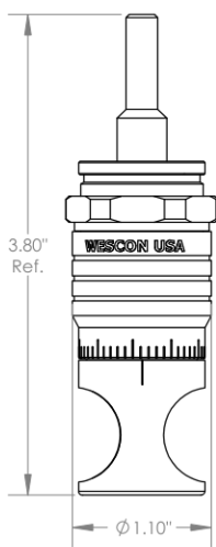
WES596-S Microstop with Ø 1/4" Standard Shaft
