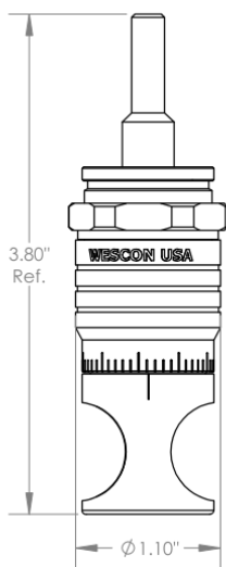
WES596-S Microstop with Ø 1/4" Standard Shaft
