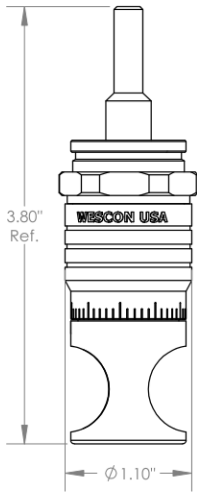
WES597-S Microstop with Ø 1/4" Standard Shaft
