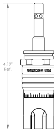
WES597-S3L-QC Microstop with Quick Change shaft
