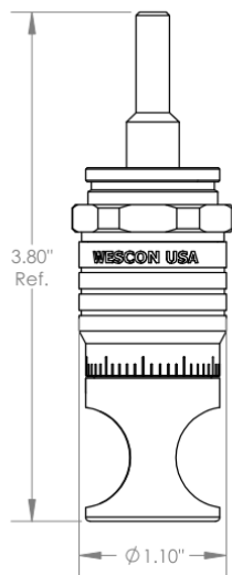
WES597-S Microstop with Ø 1/4" Standard Shaft
