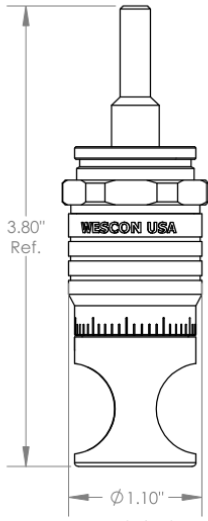
WES597-S Microstop with Ø 1/4" Standard Shaft
