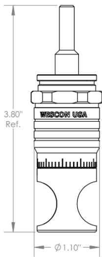
WES597-S Microstop with Ø 1/4" Standard Shaft
