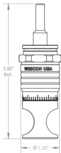
WES597-S Microstop with Ø 1/4" Standard Shaft
