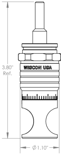
WES597-S Microstop with Ø 1/4" Standard Shaft
