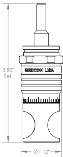
WES597-S Microstop with Ø 1/4" Standard Shaft
