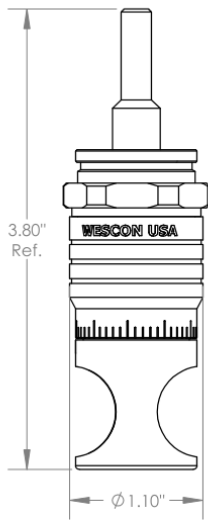
WES597-S Microstop with Ø 1/4" Standard Shaft
