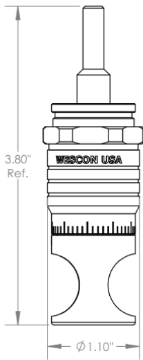
WES597-S Microstop with Ø 1/4" Standard Shaft
