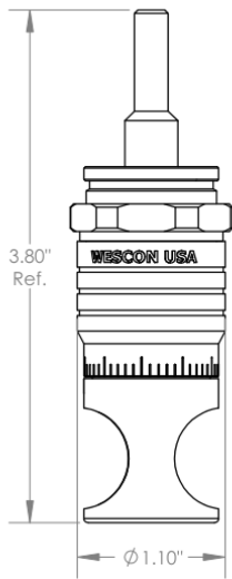
WES597-S Microstop with Ø 1/4" Standard Shaft
