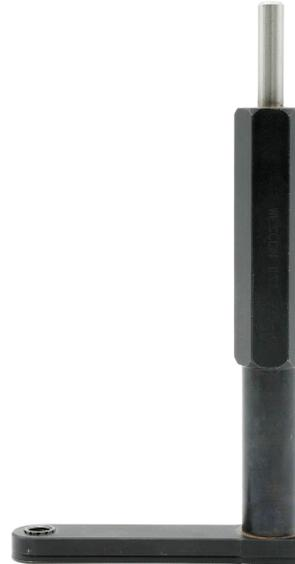
For access to very tight areas. The WES900 series is designed to fit 1/4"-28 threaded drill bits and has a 1/4" round shaft. Choose from straight, right hand, or left hand styles with various offsets. Optional tri-flats or quick change shafts are available. A 1/2" round handle is standard, with an optional 11/16" hex handle available. Also known as a L-Type drill attachment, drill offset, drill right angle attachment, pancake drill attachment, or drill offset adapter.
