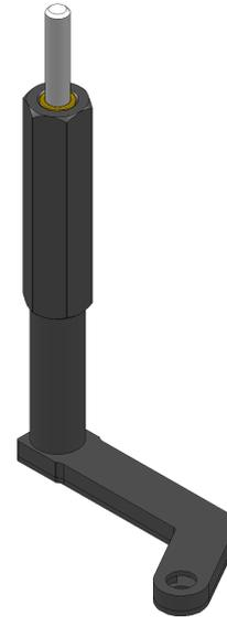
For access to very tight areas. The WES900 series is designed to fit 1/4"-28 threaded drill bits and has a 1/4" round shaft. Choose from straight, right hand, or left hand styles with various offsets. Optional tri-flats or quick change shafts are available. A 1/2" round handle is standard, with an optional 11/16" hex handle available. Also known as a L-Type drill attachment, drill offset, drill right angle attachment, pancake drill attachment, or drill offset adapter.
