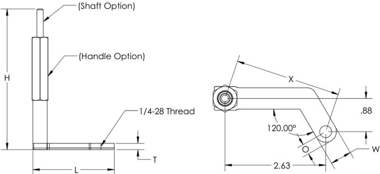
Light Duty with sleeve bearing shaft to run upto 3000 RPM
