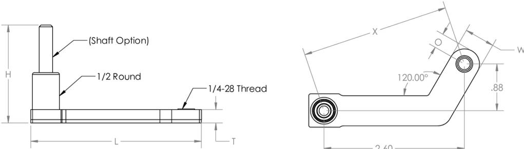
Light Duty with sleeve bearing shaft to run upto 3000 RPM
